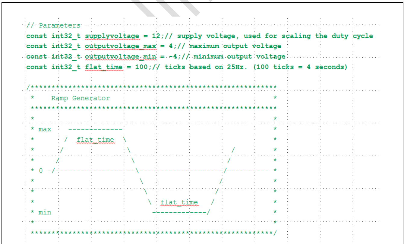
7 Figure 14 Ramp generator and its parameters
