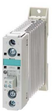
SEMI-COND. CONTACTOR 3RF2,1-PH. AC 51 20 A 40 DEGREES C 48-460 V / 110-230 V AC LOW NOISE
