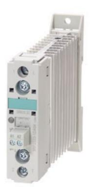
SEMI-COND. CONTACTOR 3RF2,1-PH. AC51 20 A 40 DEG. C 48-460 V / 4-30 V DC SHORT-CIRC. RESIST. WITH B-MCB
