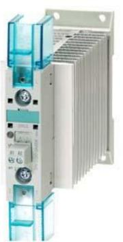
SEMICOND. RELAY 3RF2, 1-PHASE AC51 30 A 40 DEG. C 48-460 V /4-30 V DC RING CABLE CONNECTION
