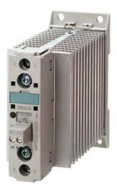
SEMI-COND. CONTACTOR 3RF2,1-PH. AC 51 30 A 40 DEGREES C 48-600 V / 24 V DC SCREW TERMINAL
