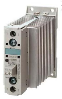
SOLID-STATE CONTACTOR 3RF2,1-PH AC51 30A 40 DEGR. C 48-600V / 110-230VAC SCREW CONNECTION BLOCKING VOLTAGE 1200V
