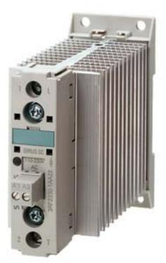
SEMI-COND. CONTACTOR 3RF2,1-PH. AC 51 30 A 40 DEGREES C 48-600 V / 110-230 V AC SCREW TERMINAL
