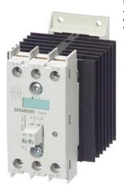
SEMI-CONDUCTOR CONTAC.3-PH.3RF2 AC51 20A 40 DEG. C 48-600V / 4-30V DC 2-PHASE CONTROLLED SCREW TERMINAL BLOCKING VOLTAGE 1200V
