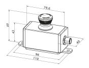
Equipped Stainless Steel Enclosure with M12 cable entry (8 poles)for profile rail mounting S41\_01
