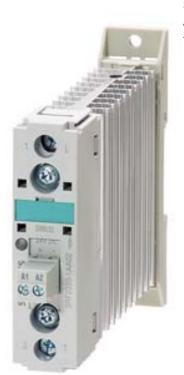
SEMI-COND. CONTACTOR 3RF2,1-PH. AC 51 20 A 40 DEGREES C 48-460 V / 110-230 V AC SCREW TERMINAL
