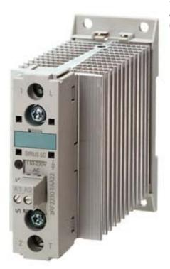
SEMI-COND. CONTACTOR 3RF2,1-PH. AC 51 30A / AC15 15A 40 DEG. C 48-460 V / 24 V DC SCREW CONNECTION INSTANTANEOUS SWITCHING
