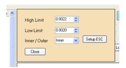
**Setup Enter**: When button is pressed, the upper/lower limit and the mode can be modified; when button is up, the settings will be sent and saved in the device.
