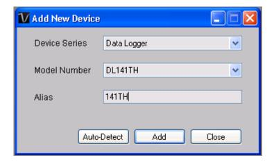
Enter a unique alias for this device, click "Add" will add the device into Voltsoft. User may also launch this module by selecting Device Management->Add New Device in menu.
