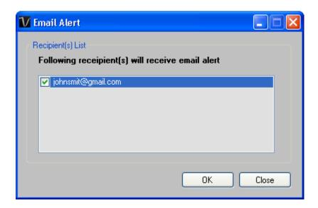
As SL451 supports real time measurement, therefore, it has an email alert feature, which will send out an email to the specified user when the device reading is above or below a certain level. The alert level can be configured in Setting.
