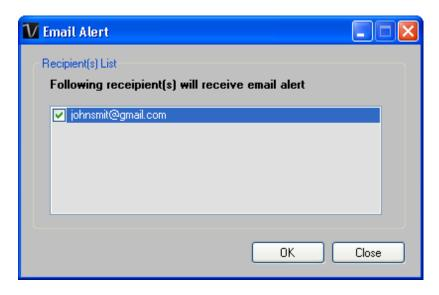
As DL161S supports real time measurement, therefore, it has an email alert feature, which will send out an email to the specified user when the device reading is above or below a certain level. The alert level can be configured in Setting.
