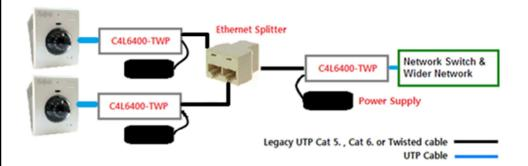
C4L6400-TWP transceivers are used to extend the Ethernet IP signals via Cat 5E, Cat 6 or 2 wire cable in the existing UTP network in building.
