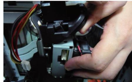
5 Pull open the quick-detachment lock to release the extruder module. Tilt the module and remove it from the slot. Provide proper safekeeping of the extruder.
