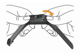
2 Insert the device into the flexible silicone clip by stretching the clip material around the device.
