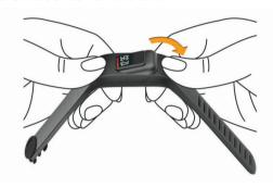
2 Insert the device into the flexible silicone band by stretching the band material around the device.
