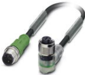
Sensor/Actuator cable, 3-position, PUR halogen-free, black-gray RAL 7021, Plug straight M12, A-coded, on Socket angled M12, A-coded, with 2 LEDs, Cable length: 3 m
