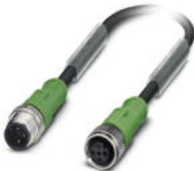
Sensor/Actuator cable, 3-position, PUR halogen-free, black-gray RAL 7021, Plug straight M12, A-coded, on Socket straight M12, A-coded, Cable length: 1.5 m
