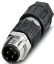
Sensor/actuator connector, Universal, 4-position, Plug straight M12, A-coded, Insulation displacement connection, Knurl material: Stainless steel, External cable diameter 3.5 mm ... 6 mm
