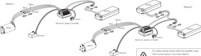
1) Picture 1 is for SEA-SERIES-30A-V3, SEA-SERIES-60A-V3 and other ESCs that work with one LiPo battery pack; that is a wiring diagram with 1 battery pack. 2) Picture 2 is for SEA-SERIES-120A-V3. SEA-SERIES-180A-V3. SEA-SERIES-130A-HV-V3 (without switch) and other ESCs that may work with two LiPo battery packs; that is the wiring diagram with 2 battery packs.
