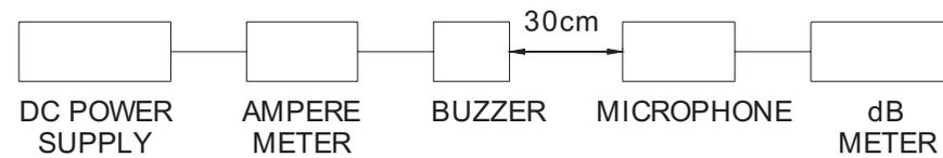
In the measuring test, buzzer is placed as follows:
