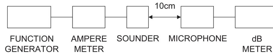
In the measuring test, buzzer is placed as follows:
