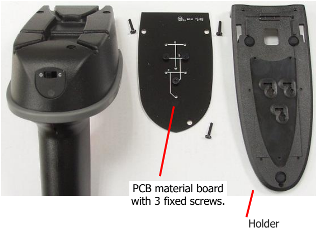
PCB material board with 3 fixed screws.
