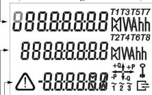
Auxiliary display 1 (active power\* in kW or MW) (M2/M3: reactive energy or power in kVAr(h) or MVAr(h)\*) Auxiliary display 2 (e.g. IN, OUT for import or export) In case of error: error code alternates with current display \* EM238x transformer meter: CT and VT are taken into account Power: negative sign for export
