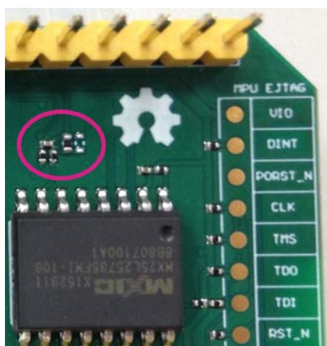
Figure 8 JTAG resistors on LinkIt Smart 7688 Duo bottom view
