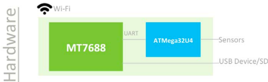
Figure 44 LinkIt Smart 7688 Duo Hardware Architecture
