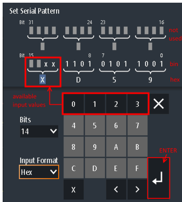
Figure 3-17: Pattern editor for 14-bit pattern in hexadecimal format
