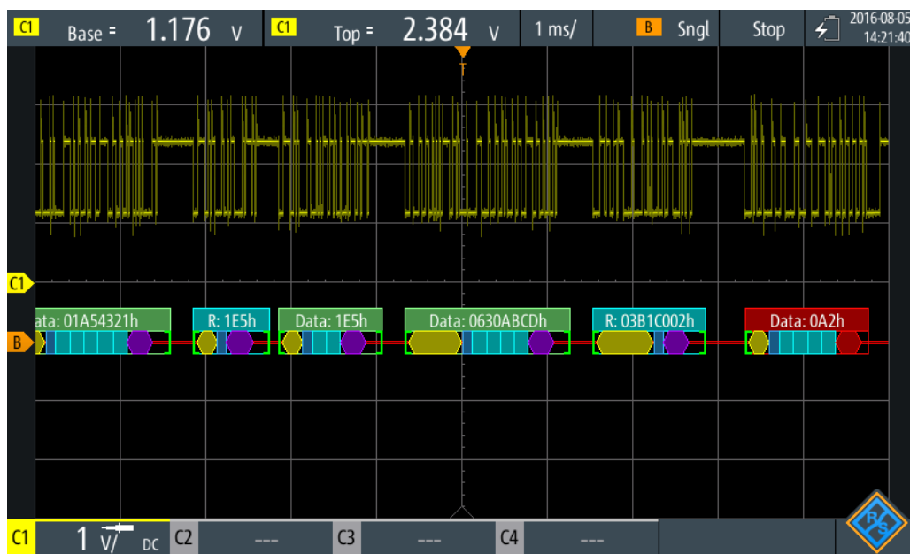
Figure 9-30: Comb display of a decoded CAN signal, triggered on address 0630ABCD (hex)
