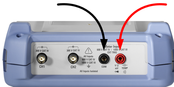
Figure 7-1: Meter inputs to connect test leads
