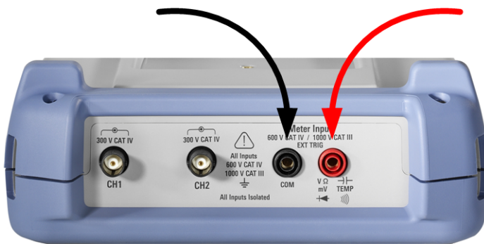
Figure 4-1: Meter inputs to connect test leads
