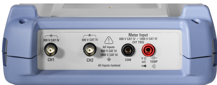
Figure 3-3: Top view of R&S RTH1002
