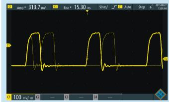
The high-speed acquisition system of the R&S®ScopeRider captures up to 50 000 waveforms/s and uncovers rare and unexpected signal
