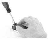
Then screw the 2 screws at the opposite side tight. However, make sure that the screws are not screwed in too tightly, to avoid damaging the thread.
