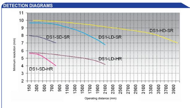
Variation of the minimum resolution according to the operating distance between the emitting and receiving units.
