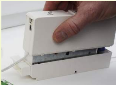
Fig. 29: Connecting the upper housing with the lower
