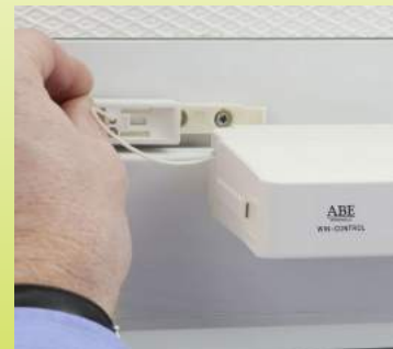
Fig. 36: Removing the clip (A1)
