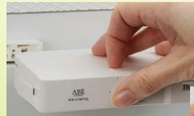
Fig. 38 / 39: Removing the bracket
