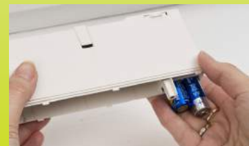
Fig. 40: Removing the batteries
