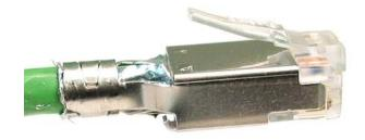
18 Crimp contacts and shield fingers. Trim off excess shield
