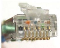
Verify wires are visible through end of plug
