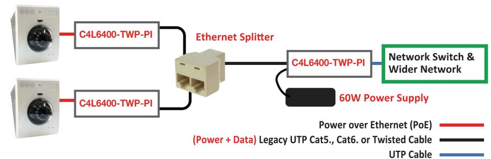
**C4L6400-TWP-PI** transceivers are used to extend the Ethernet IP signals via Cat 5E, Cat 6 or 2 wire cable in the existing UTP network in building.
