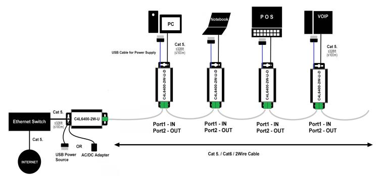
C4L6400-2W-U-D transceivers are used to extend the Ethernet IP signals via 2Wire cable in the existing 2Wire network in building.
