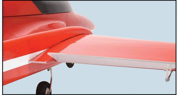
🇬🇧 Elevator: 20mm each way at tip of elevator, with 35% exponential.
