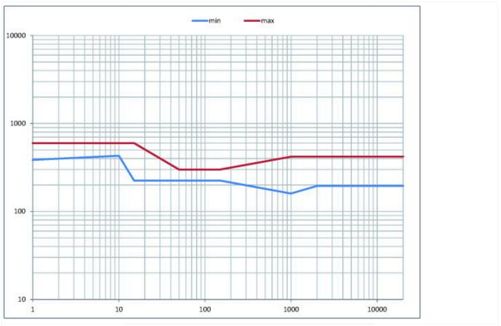
Tripping current frequency range: | FRCdM, 300 mA, type B+
