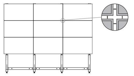
Note: A 1.27 mm gap between bezels is recommended for heat expansions.
