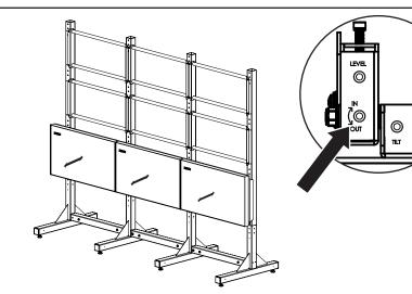
Now that you have your first lower center display attached to the frame, the beauty of the three part alignment features of the mounting bracket come into play. The fact that all the adjustments are on top will make the final adjusting effortless.
