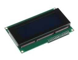
This 20x4 character LCD suits perfectly for your project. It works with a PCF8574 adapter chip and a blue backlight. Moreover, it is conforming to the HD44780 industrial standard.
