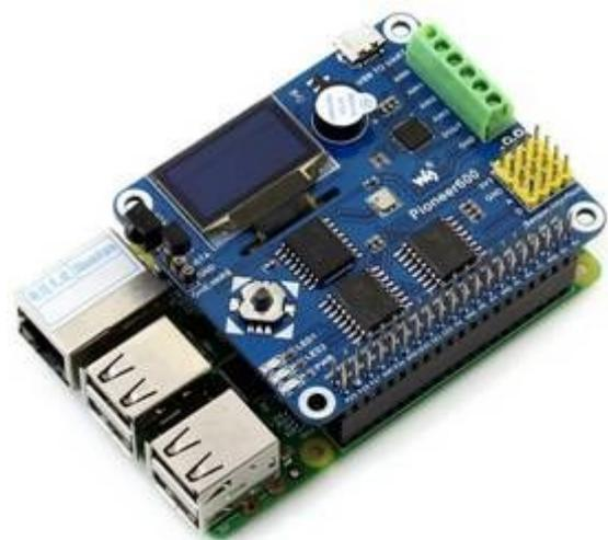
Connected to Raspberry Pi B+/2/
