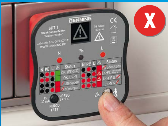
Socket with wiring error, danger to life! External conductor (L) and protective conductor (PE) have been inverted!
