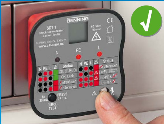
Socket is installed correctly, contact sensor checks the PE contact for dangerous contact voltage
