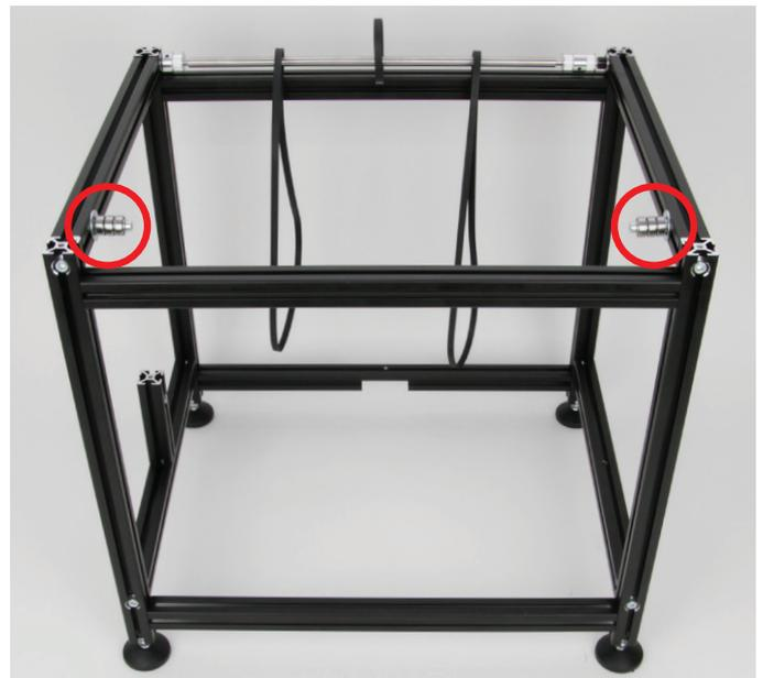
Push one slot nut each into the inside of the upper aluminium profiles of the side parts and attach one belt tensioner each to it. Do not tighten the screws firmly yet.
