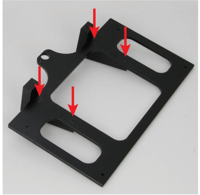
Attach the two table tappets with the 4 recessed-head screws to the undertable from below. The recessed bores in the undertable must be on top. Optionally, the screws can be secured with threadlocker varnish.
