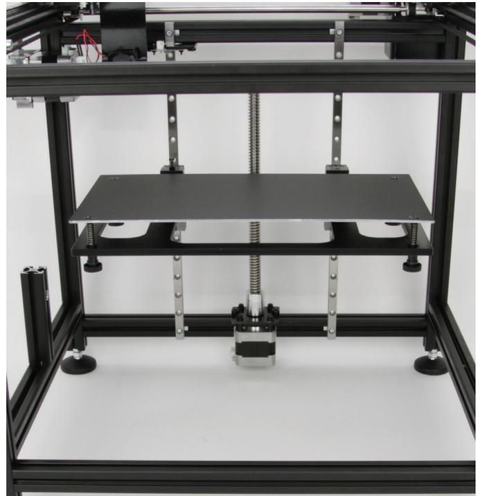
Insert one screw at a time and guide them through the bores in the undertable.
