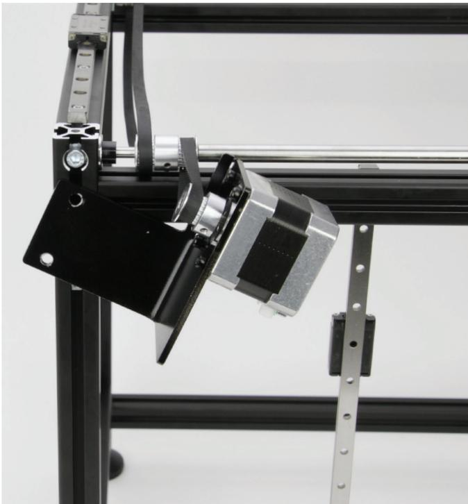
Attach the sprocket of the motor as shown in the figure to the short toothed belt of the deflection shaft.
