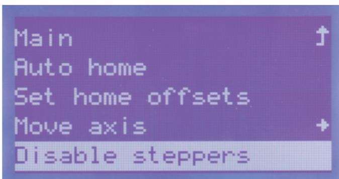
Go to the menu "Prepare" and navigate to item "Disable steppers". Push the button of the operating knob (10). By this, all motors are switched off so you can move the X and Y axes manually.
