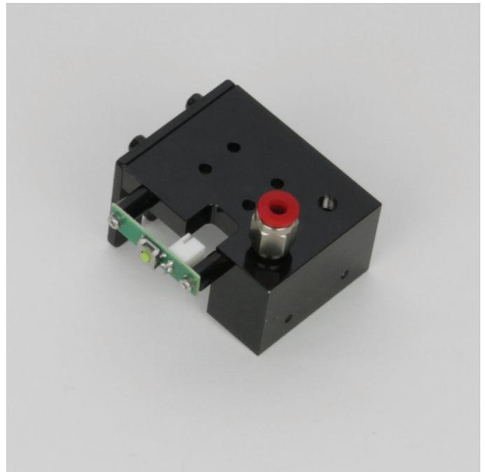
Mount the limit switch PCB on the extruder holder with the two cylinder-head screws M2x16 on the left, at the cut-out. A spacer must be used between each extruder holder and the limit switch PCB. Optionally, the screws can be secured with threadlocker varnish.
