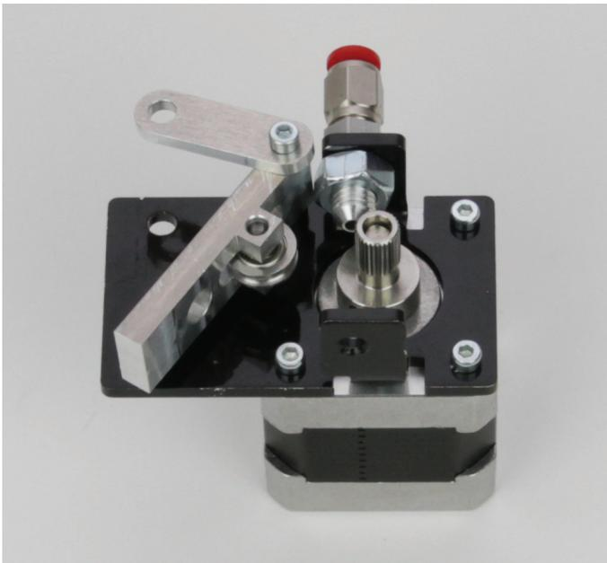
Install the unit previously assembled in the free bore of the motor.
