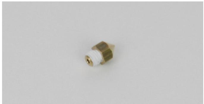
Cut about 2 to 3 cm thread sealing tape off of the roll and wind it around the thread of the nozzle. Cut off the sealing tape that protrudes over the thread with a sharp knife, e.g. by running the knife along the upper-most groove of the thread.
