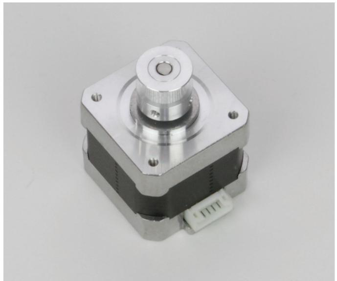
Push sprocket onto axle of the actuator and attach it with 2 threaded pins each. A threaded pin must meet the flattened side of the axis. The motor axis must end flush with the upper edge of the sprocket. Optionally, the threaded rods can be secured with threadlocker varnish.
