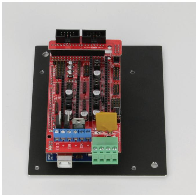
Push the additional PCB onto the main PCB.
