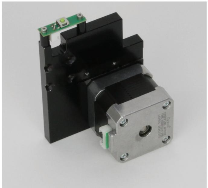
Install a limit switch PCB with the two cylinder-head screws M2x16 at the right guide carriage plate.
