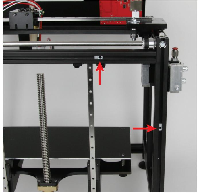
Push the 2 slot nuts into the groove of the upper aluminium profile and the left aluminium profile (viewed from the front) at the rear as shown in the figure. The threads must be aligned to the right or downwards as illustrated.
