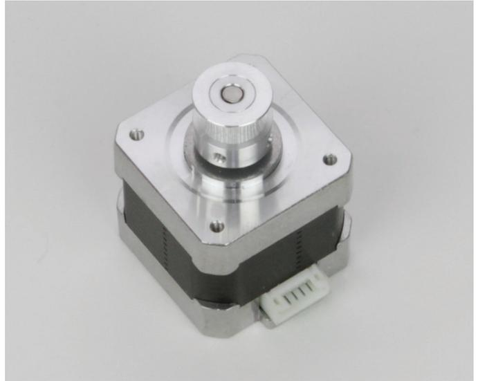
Push sprocket onto axle of the actuator and attach it with 2 threaded pins each. A threaded pin must meet the flattened side of the axis. Do not tighten the threaded pins fully yet. The motor axis must end flush with the upper edge of the sprocket. Optionally, the threaded rods can be secured with threadlocker varnish.
