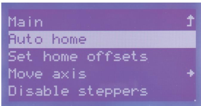
Turn the operating knob (10) until the menu item "Auto home" is selected. Push the button of the operating knob (10). All axes move into the home position.
