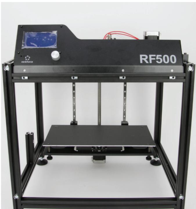
Hold the display unit against the slot nuts from above and align them with the bores in the display unit.
