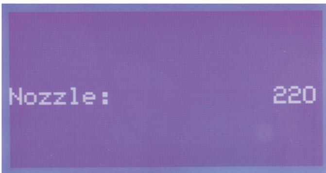
Turn the operating knob (10) to the right until the desired value "**220**" (here: 220 °C) is displayed. The extruder is heated up at once after turning.
