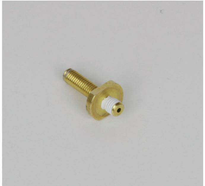
Cut about 2 to 3 cm thread sealing tape off of the roll and wind it around the short thread of the nozzle stock. Cut off the sealing tape that protrudes over the thread with a sharp knife, e.g. by running the knife along the upper-most groove of the thread.
