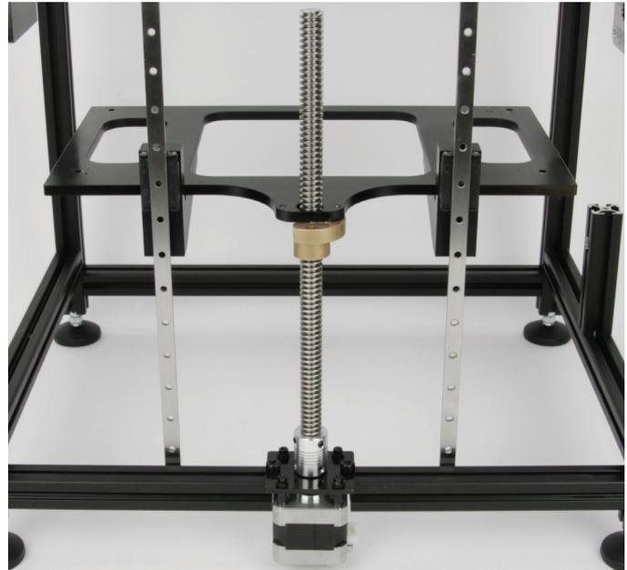
Important! The coupling level must be adjusted so that it has a distance of about 0.5 to 1 mm from the motor holding plate.
