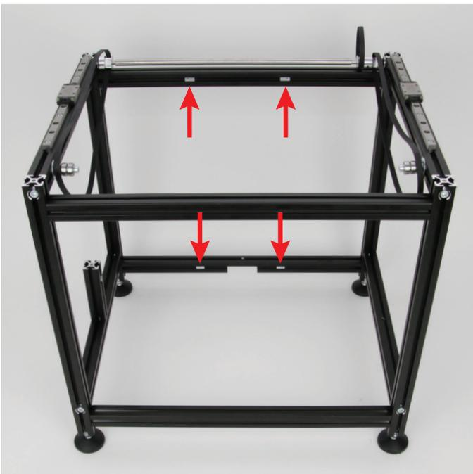
Push 2 slot nuts each into the two aluminium profiles installed cross-wise at the rear as illustrated. The slot nuts each must be aligned with the parallel bore.
