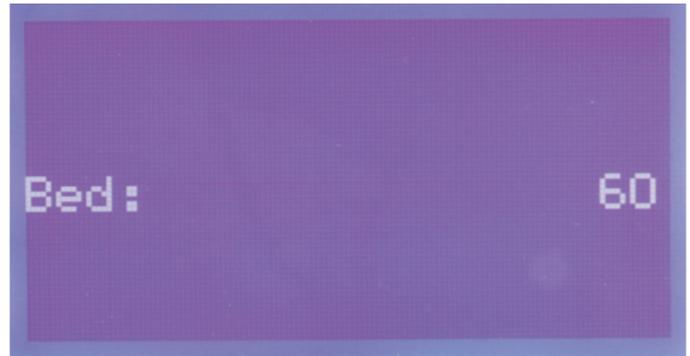
Turn the operating knob (10) to the right until the desired value "**60**" (here: 60 °C) is displayed. The heating element is heated up at once after turning.
