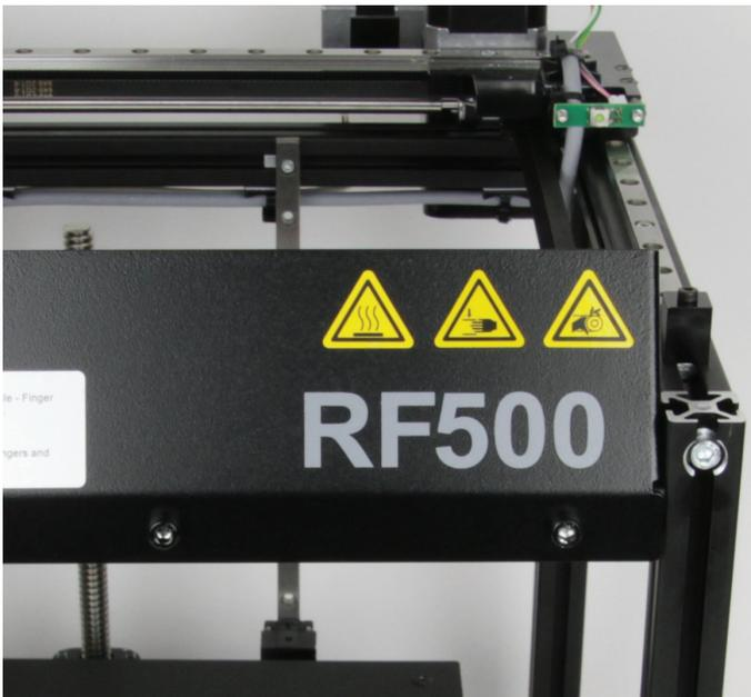
Attach the 3 yellow warning sign stickers "Hot surface", "Danger of hand injury" and "Danger of crushing" well visibly to the front cover above the "RF500" script. Degrease the adhesive areas first.
