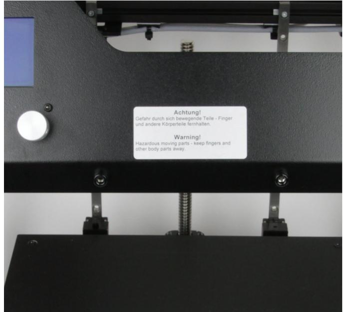
Attach the silver warning text sign well visibly to the middle of the front cover as illustrated. Degrease the adhesive area first.
