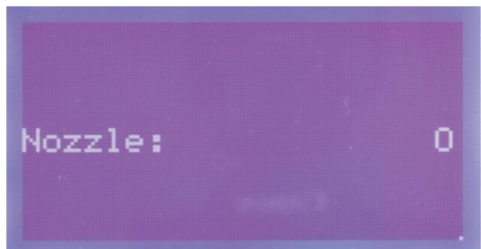
Turn the operating knob (10) to the left until the value is set to 0. The heating of the extruder is switched off by this.
