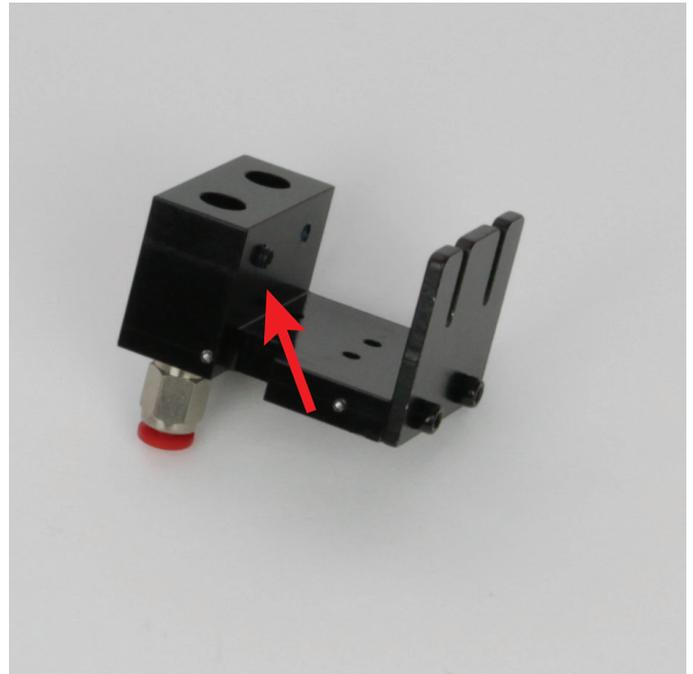
Screw the threaded pin into the bore by the quick closure from behind. Only screw in the threaded pin loosely. It must not protrude into the bore for the extruder yet.
