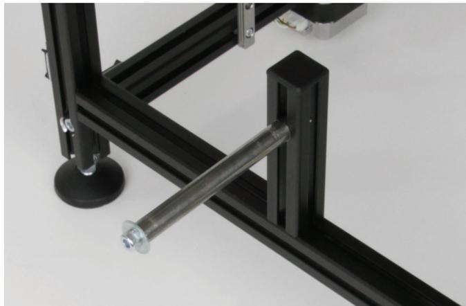
Attach the filament holder to the short aluminium profile from the inside with the cylinder-head screw M5x20.
