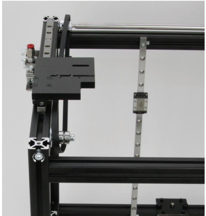
Install the left guide carriage plate with the 4 recessed-head screws on the guide carriage of the left Y-guide rail.
