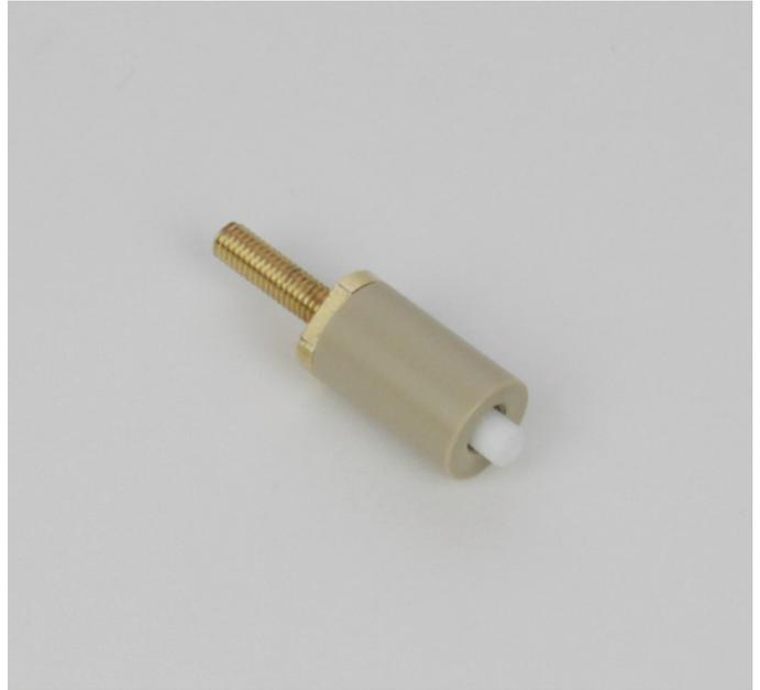
Push the PTFE insert into the PEEK part. Take a hexagon socket wrench with at least 3 mm and push the PTFE insert entirely into the PEEK part.
