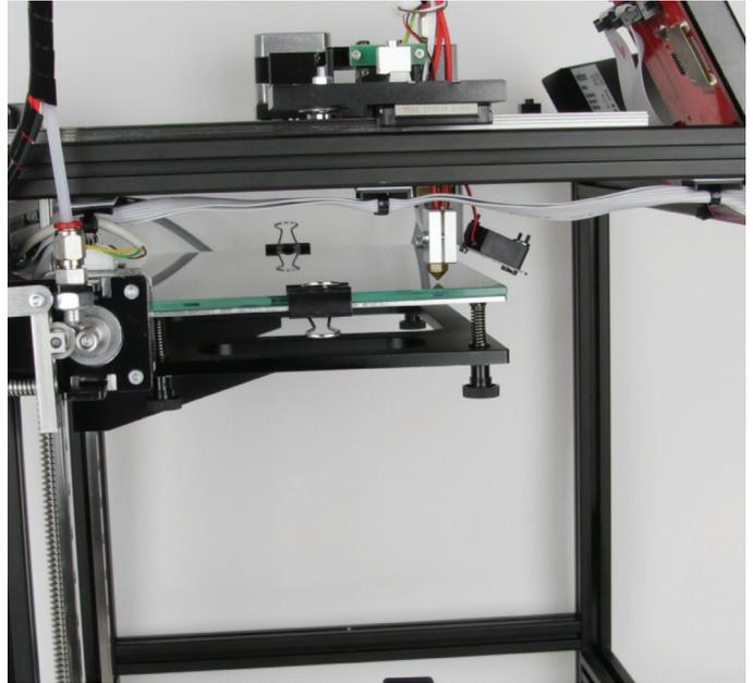
The 4 knurled nuts at the bottom of the table can be used to adjust the printing plate.
