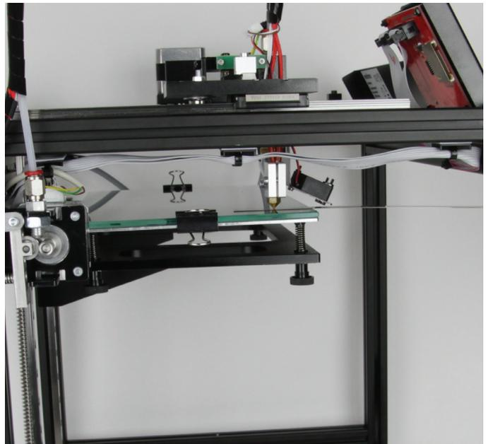
Set a distance of 0.3 mm (feeler gauge) everywhere between the nozzle and the printing plate support for the printing plate and the nozzle. Start at the point with the largest distance and proceed in sequence.
