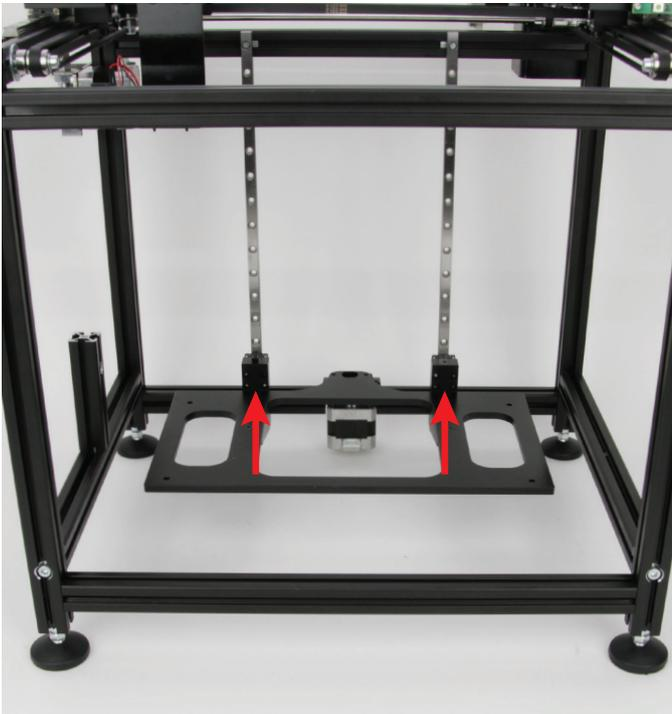
Loosely attach the table to the two guide carriages on either side with 4 cylinder-head screws. Optionally, the screws can be secured with threadlocker varnish.
