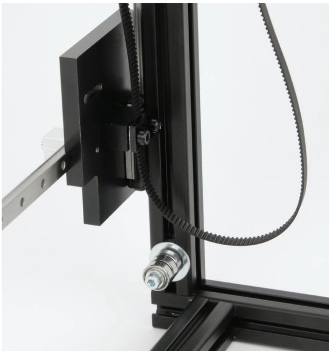
Attach the toothed belt to the bottom of the left guide carriage plate as illustrated.
