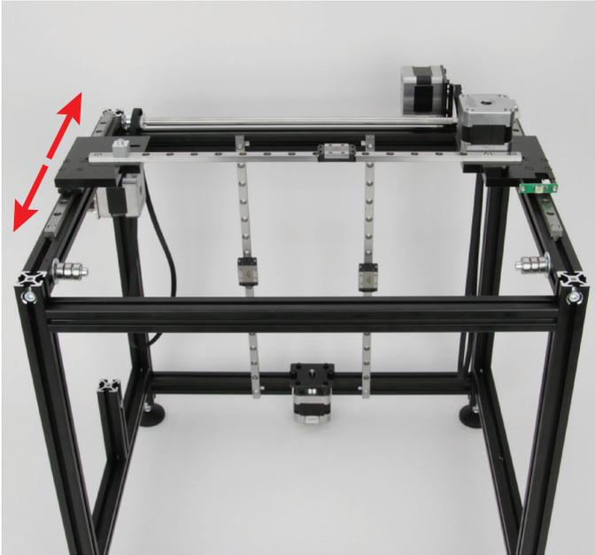
Move the X-guide rail forward and back in the Y-direction several times.
