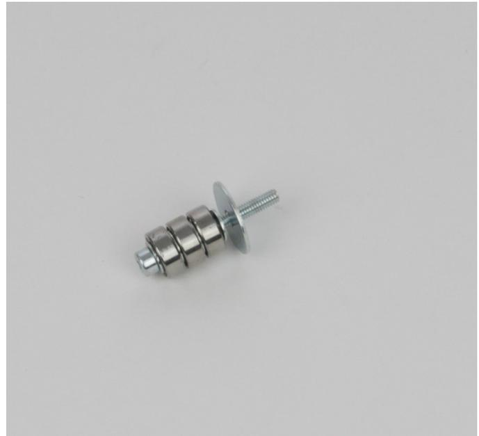
Push the washers onto the screw alternatingly with the ball bearings (screw - washer - ball bearing - washer - ball bearing - washer - ball bearing - washer - washer 20 mm).
