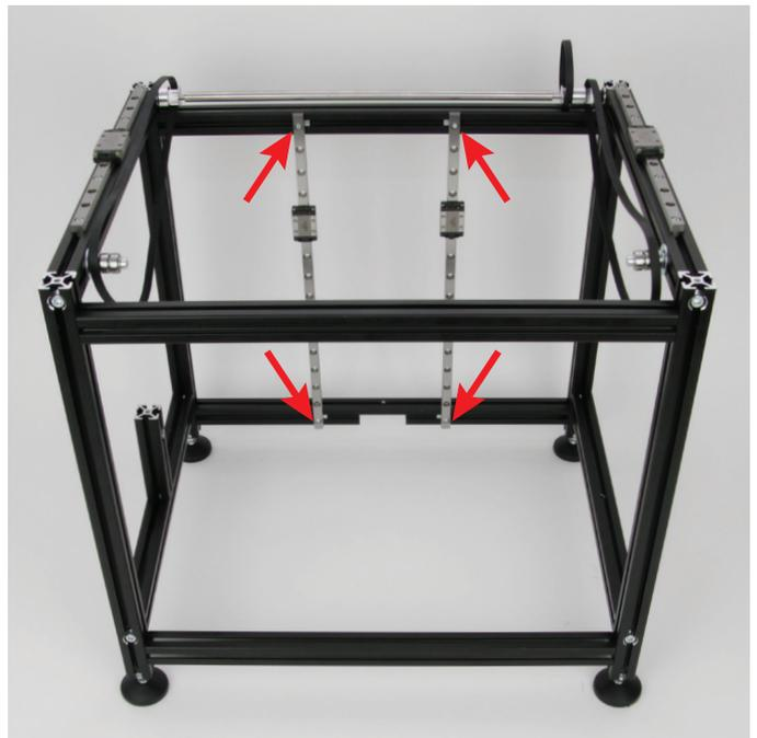
Attach the two guide rails with guide carriage to the two profiles, using the cylinder-head screws as illustrated. Only tighten the 4 screws slightly!
