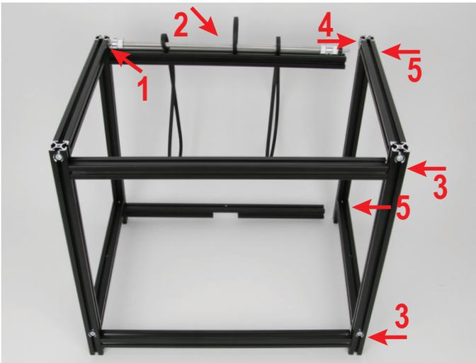
Take the assembled deflection shaft and push it into the ball bearing of the left side part (1). The three toothed belts are now simply pushed onto the shaft (2). The small toothed belt must be centred. Now attach the right side part loosely to the two front aluminium profiles (3) with 2 cylinder-head screws. Then push the deflection shaft into the ball bearing of the right side part (4). Finally, attach the right side part to the two rear profiles (5).
