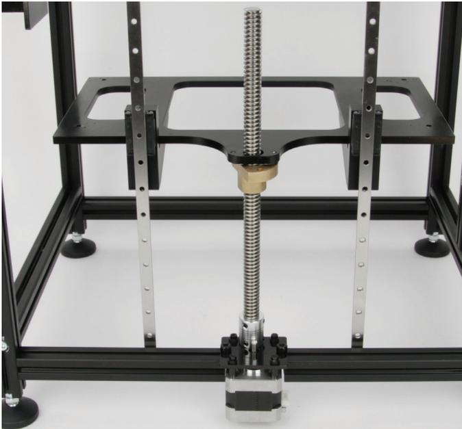
The flange nut on the spindle should be roughly centred. Move the table up and thread the spindle through the table bore from below.
