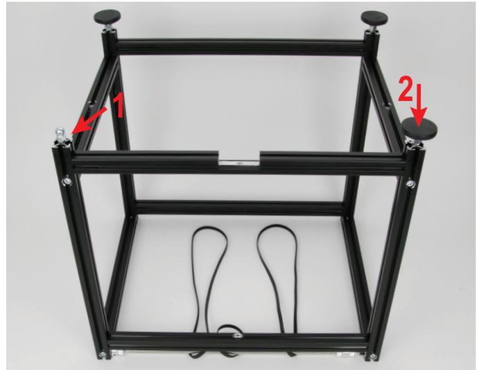
Screw the counter-nut to the stop in all four ball-head screws. Take the basic frame and put it upside-down. Do not crush the toothed belts. Screw one ball-head screw each into the bottom of the vertical aluminium profiles (1). Screw the screws in to the stop. Push one foot onto each ball head with the ball of your thumb (2). Finally, align the feet. Place the basic frame on a level, straight surface. After setting the feet, tighten the counter-nut towards the aluminium profile.
