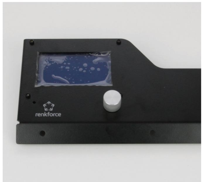
Push the operating button onto the shaft of the dial switch and attach it by tightening the slotted screw.
