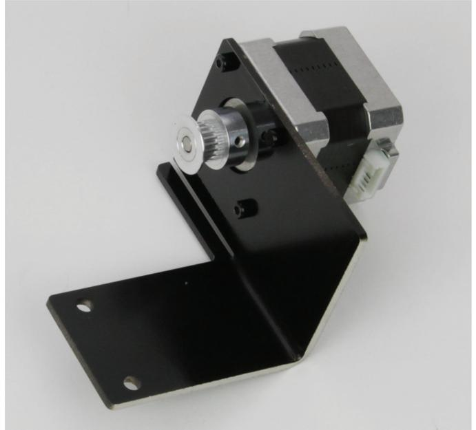
Install the motor to the Y-motor holder with the 4 M3-cylinder-head screws. The motor plug must be aligned as shown in the figure.
