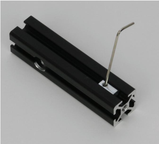
Turn the slot nut up until it "latches" and is held cleanly in the guide. Now you can move it back and forth as desired. When you tighten the respective screw in the slot nut, always make sure that the slot nut is placed cleanly in the nut.
