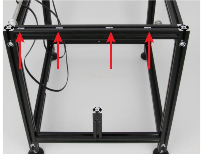
Push 4 slot nuts into the upper aluminium profiles of the two respective side parts 4 slot nuts. For the other ones, the thread must point outwards in each case.
