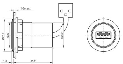
10MAX: means the panel thickness, the max thickness for the panel no more than 10mm.
