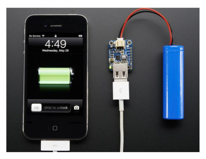
Great for powering your robot, Arduino project, single-board-computer such as Raspberry Pi or BeagleBone! Each order comes with one fully assembled and tested PCB and a loose USB A jack. If you are powering your project from USB, solder the USB A jack in (a 3-minute soldering task). If you would like to use a terminal block, pick up a 3.5mm 2pin block here (http://adafru.it/duR) and solder to the output spot where the USB jack would go. Or dont solder anything in for a more compact power pack.
