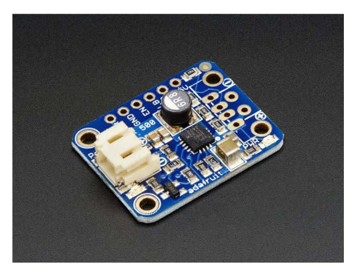
The PowerBoost 500 (http://adafru.it/dFq) has at the heart a TPS61090 boost converter from TI (http://adafru.it/duQ). This boost converter chip has some really nice extras such as low battery detection, 2A internal switch, synchronous conversion, excellent efficiency, and 700KHz high-frequency operation. Check out these specs!
