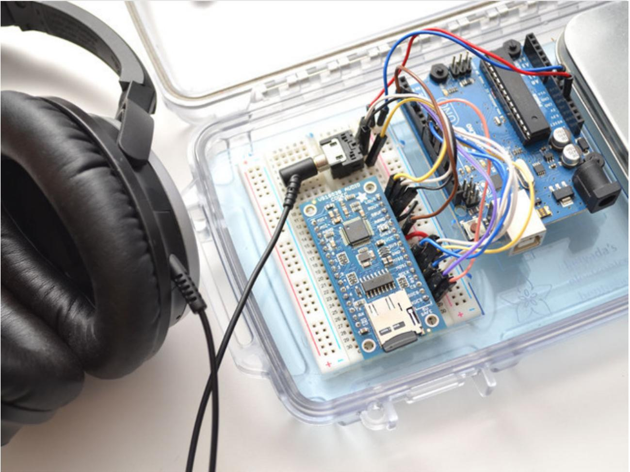
The VS1053 can be configured as a simple audio player under control of the Arduino. The Arduino reads data from the on-board SD card, then plays it back through the CODEC via the SPI interface.
