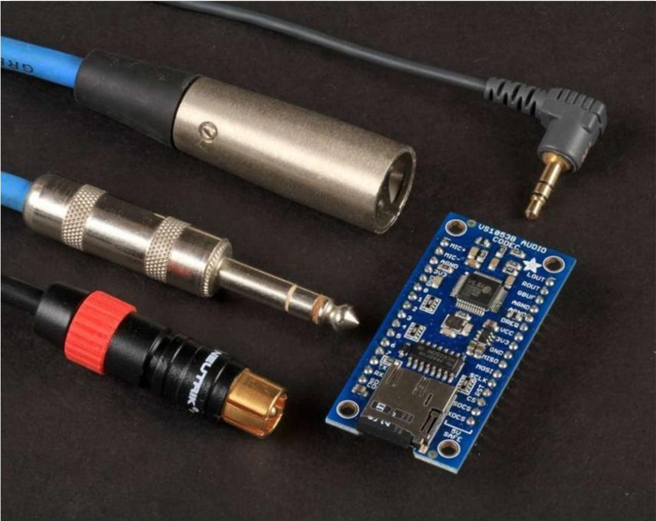
Both the VS1053 version 1 (shown above, does not have big round silver capacitors at the top) **and** the version 2 (has a v2 label, has two big round silver caps) can drive a pair of headphones directly. Just connect the LOUT and ROUT to the left and right pins of the headphone jack. The center pin should be connected to GBUF.
