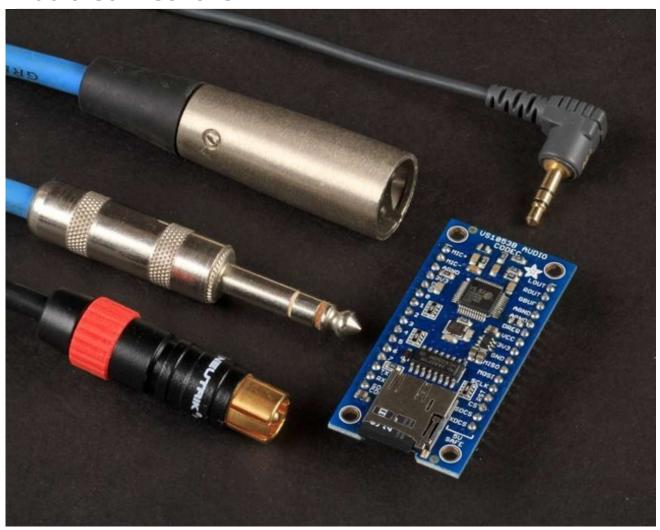
Both the VS1053 version 1 (shown above, does not have big round silver capacitors at the top) **and** the version 2 (has a v2 label, has two big round silver caps) can drive a pair of headphones directly. Just connect the LOUT and ROUT to the left and right pins of the headphone jack. The center pin should be connected to GBUF.
