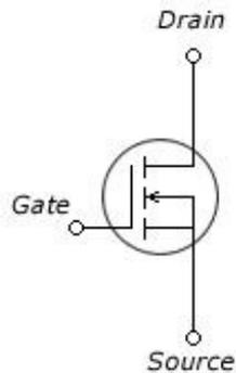
Internally, the "Source" of the FET is connected to Ground. But the Drain is left open. When switched on, the FET provides a path for current to flow from the output pin to ground.
