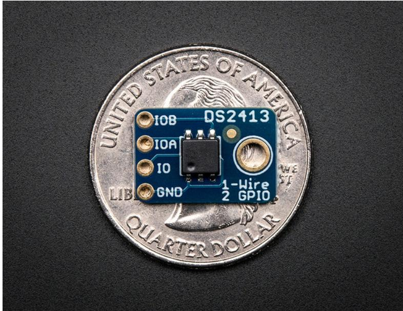
Pins are precious in the microcontroller world. How many times have you needed just one more pin? Sure, you could step up to a Mega and get a whole bunch more, but what if you really just need one or two? The DS2413 breakout board is the perfect solution. Each DS2413 breakout has 2 open drain GPIO pins and a 1-Wire interface. Just one of these boards will give you 2 pins for the price of one. But you can keep expanding from there.
