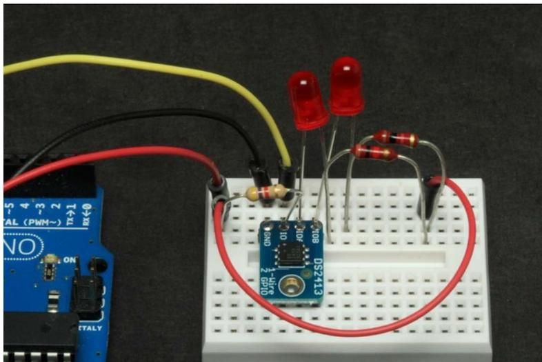
Compile and upload the example sketch and you should see both LEDs blinking: 1 second on and 1 second off.
