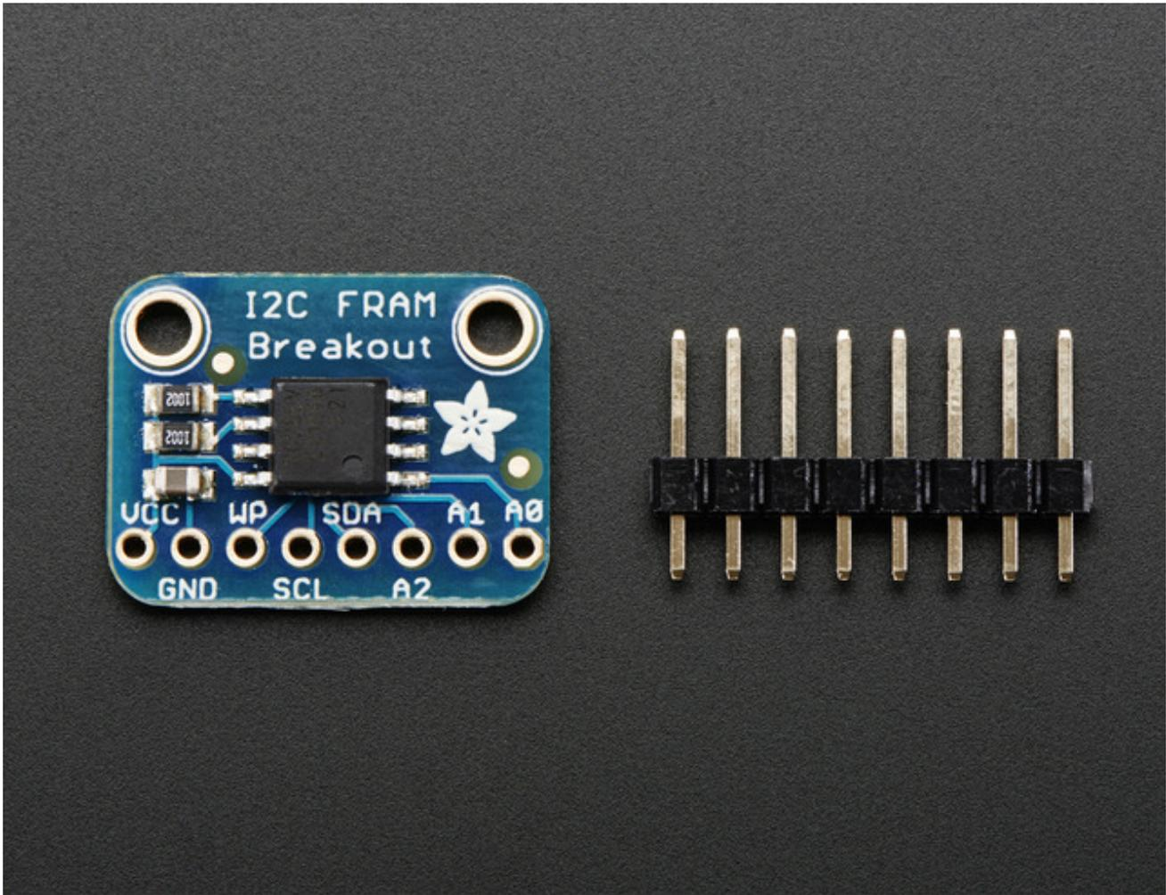
This particular FRAM chip has 256 Kbits (32 KBytes) of storage, interfaces using I2C, and can run at up to 1MHz I2C rates. Each byte can be read and written instantaneously (like SRAM) but will keep the memory for 95 years at room temperature. Each byte can be read/written 10,000,000,000,000 times so you don't have to worry too much about wear leveling.
