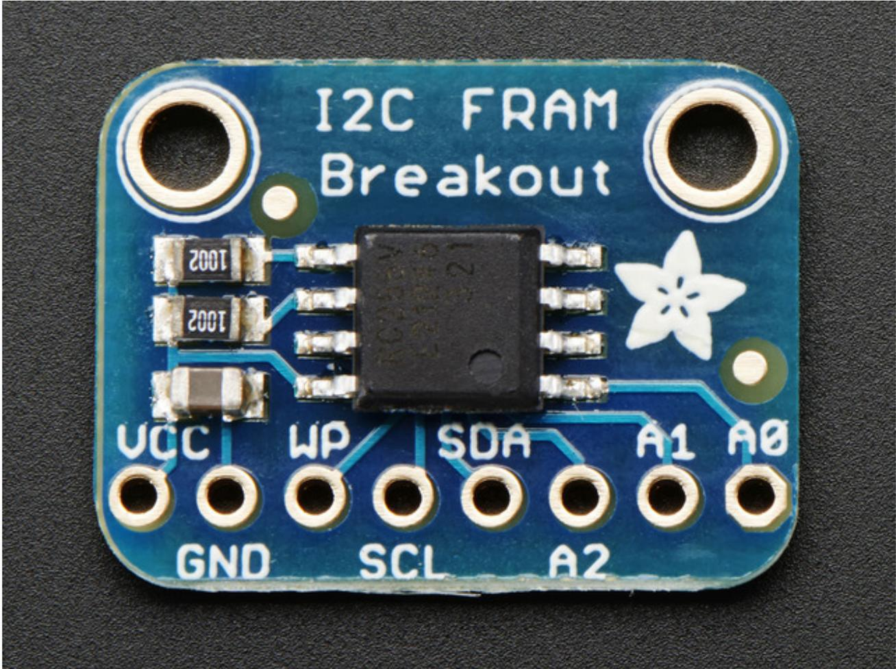
The FRAM chip is the little guy in the middle. On the bottom we have the power and interface pins
