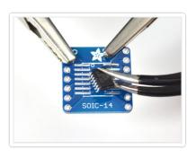
Next you need to place the part onto the pads, and you'll want to get the orientation right. You can look for a dot (indicating pin #1). In some cases, look for a flattened corner (on the left side here) which indicates which side is on the left
