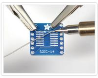
We'll start by melting a little solder on one corner pad. I like going with the top right corner. Melt just a tiny bit on, so its rounded but not blobby
