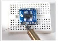
Almost done, now all you have to do is solder each header pin into the corresponding hole to make a secure connection
