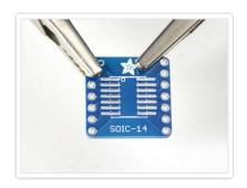
Begin by placing the breakout adapter into your vise/third hand to keep it steady.
