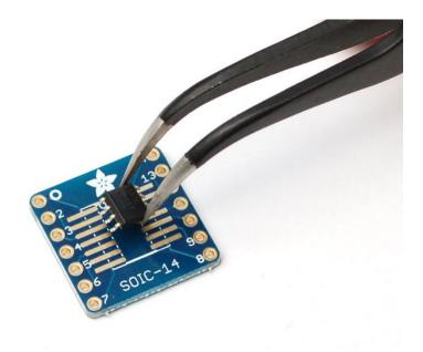
Nothing is as fast and fun as prototyping on a breadboard, but at some point you will find that the chips you want to work with are only available in non-breadboard-friendly SMT/SMD (Surface Mount Technology/Surface Mount Device). Unlike most DIP chips and resistors, SMT parts do not have the leads going through holes in the PCB. Instead, they 'float' on top, with often-rectangular solder pads.
