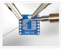
We'll start by melting a little solder on one corner pad. I like going with the top right corner. Melt just a tiny bit on, so its rounded but not blobby
