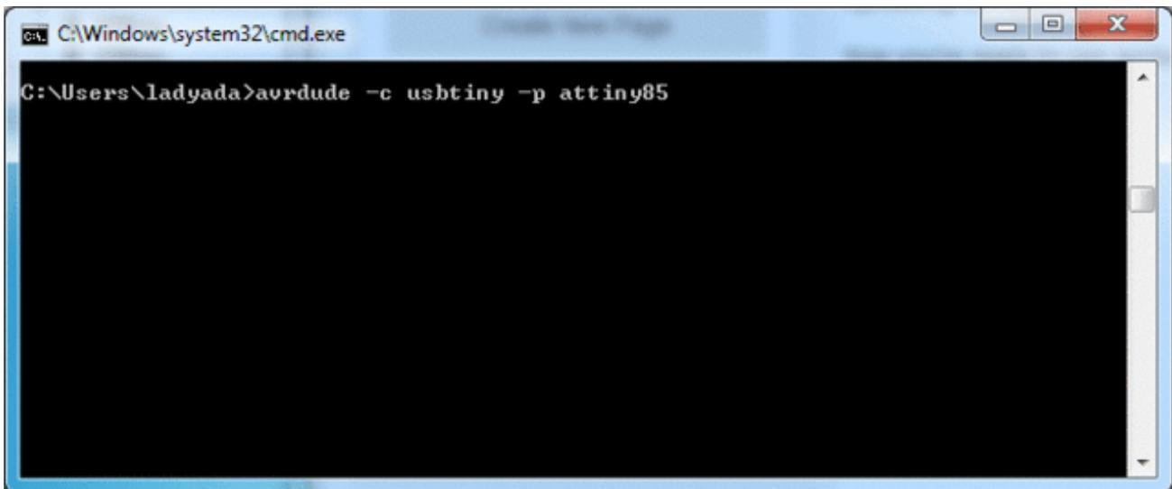
Now plug in the Trinket into the computer's USB port and/or press the reset button to enter the bootloader. You should see the red LED pulsing. Now press return, you should get the same
