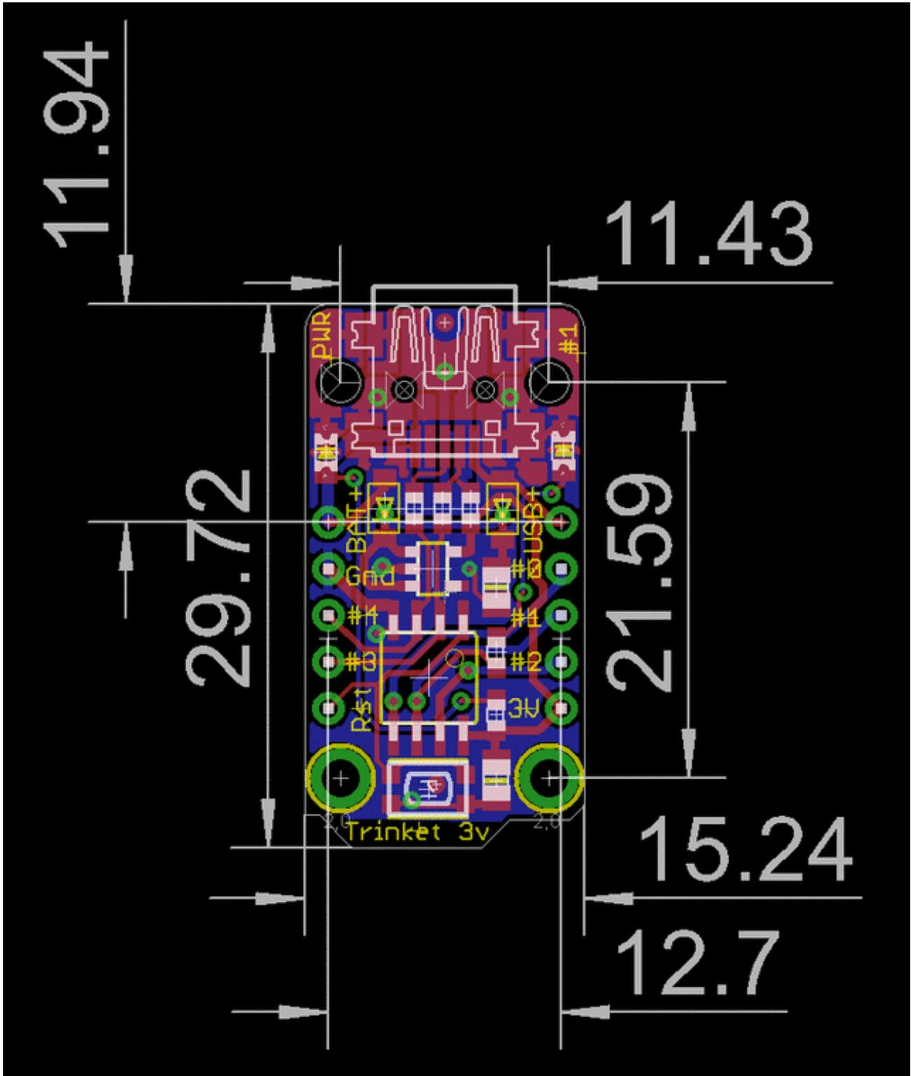
There are two versions of the Trinket: 3V and 5V. They are almost identical but there are slight differences in the pinouts: one has a 3V output pin in the bottom right, the other has a 5V output pin instead
