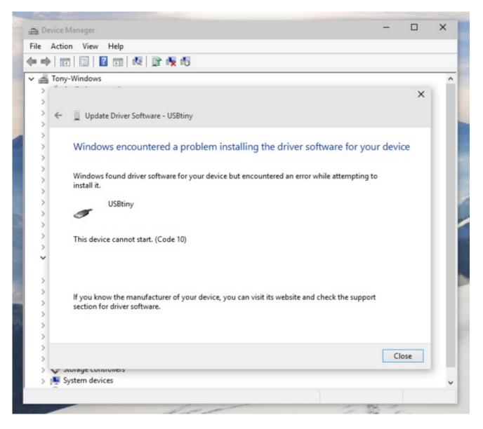
Don't worry! This just means the Trinket/Gemma bootloader timed-out before the driver finished installing. Everything should still be fine and you can continue along with the installation. Click **Close** to finish the install.
