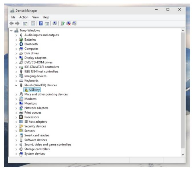
Don't worry if the device has an exclamation point next to it indicating a problem. Press the Trinket/Gemma bootloader button and after a moment device manager should update to show the device is working:
