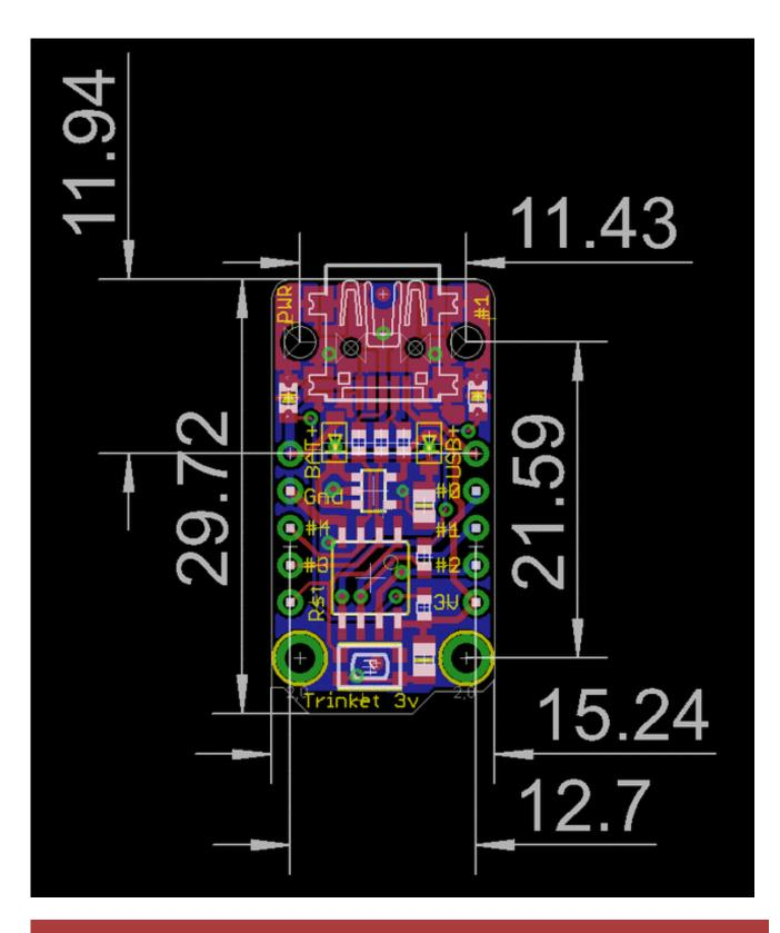
There are two versions of the Trinket: 3V and 5V. They are almost identical but there are slight differences in the pinouts: one has a 3V output pin in the bottom right, the other has a 5V output pin instead
