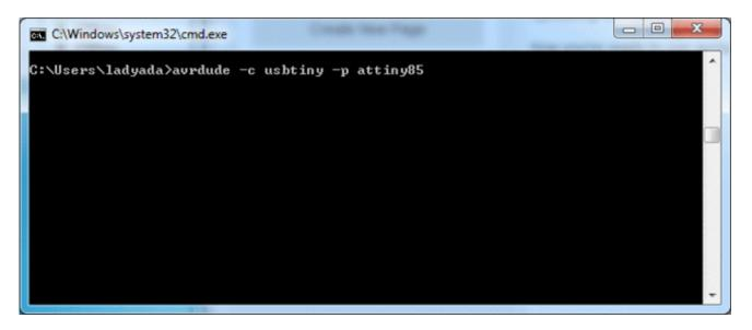
Now plug in the Trinket into the computer's USB port and/or press the reset button to enter the bootloader. You should see the red LED pulsing. Now press return, you should get the same
